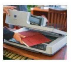
6. As shown in the accompanying figure, a(n) \_\_\_\_\_\_ is an input device that captures printed text and graphics and transfers them to a computer in digital form
