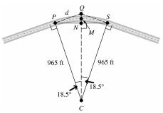
To find the distance between P and Q, d, we first note that angle QPC is a right angle. Hence, triangle QPC is a right triangle and we can solve
