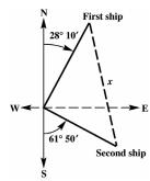
The angle between the bearings of the ships is  $180^{\circ} - (28^{\circ}10' + 61^{\circ}50') = 90^{\circ}$ . The triangle formed is a right triangle. The distance traveled at 24.0 mph is (4 hr) (24.0 mph) = 96 mi. The distance traveled at 28.0 mph is (4 hr)(28.0 mph) = 112 mi.
