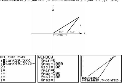
The height of the triangle is 433 ft. (rounded to three significant digits)
