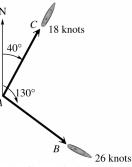
Since d = rt, the distance traveled by the first ship in 1.5 hr is (1.5 hr)(18 knots) = 27 nautical mi and the second ship is (1.5hr)(26 knots) = 39 nautical mi.
