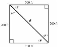
By the Pythagorean theorem,  $700^2 + 700^2 = d^2 \Rightarrow 2.700^2 = d^2 \Rightarrow d = \sqrt{2.700^2} \Rightarrow d = 700\sqrt{2}$ . Thus, length of the diagonal is  $700\sqrt{2}$  ft. To to find the angle,  $\theta$ , we consider the following isosceles triangle.
