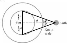
Since the included angle is 32',  $\frac{1}{2}(32')=16'$ . We will use this angle, d, and half of the diameter to set up the following equation.
