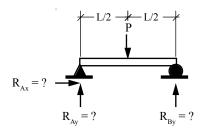
$$\sum_{\substack{(R_{By} * L) - (P * L/2) = 0 \\ R_{By} * L = PL/2 \\ R_{By} = P/2 \uparrow} \sum_{\substack{(R_{Ay} + R_{By} - P = 0 \\ R_{Ay} = P - R_{By} \\ R_{Ay} = P - P/2 \\ R_{Ay} = P/2 \uparrow$$
