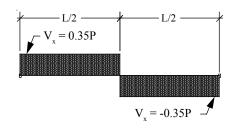
$$\begin{array}{lll} R_{_{Ax}} &=& 0 \\ R_{_{Ay}} &=& P/2 \;\; (upward) \\ R_{_{By}} &=& P/2 \;\; (upward) \end{array}$$
