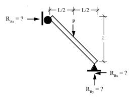
$$\sum_{\substack{(P * L/2) - (R_{Ax} * h) = 0 \\ (R_{Ax} * h) = PL/2 \\ R_{Ax} = PL/2h \rightarrow}} \sum_{\substack{F_X = 0 \\ R_{Ax} + R_{Bx} = 0 \\ R_{Bx} = - R_{Ax} \\ R_{Bx} = PL/2h}$$
