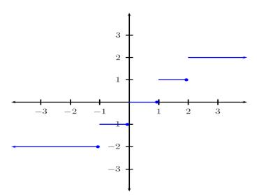
The system is i) memoryless, ii) not invertible (any input greater than 2 goes to the same output (2)), iii) causal, iv) stable, v) time invariant, vi) not linear  $(x_1(t) = 2 \to 1 \text{ and } x_2(t) = 1 \to 0 \text{ but } x_1(t) + x_2(t) \to 2 \neq 1 + 0.$
