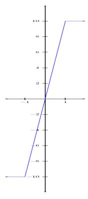
The system is i) memoryless, ii) not invertible (output = 10 for all input values > 10, iii) causal, iv) stable ( $|y(t)| \le 10$  for any input), v) time invariant, vi) not linear (suppose x(t) = 3 then y(t) = 3 but 4x(t) has output  $10 \ne 3(4) = 12$ .
