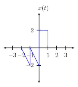
The plot of  $x_o(t)$  is determined by  $x_o(-t) = -x_o(t)$ , the plot of  $x_e(t)$  is determined by  $x_e(t) = x(t) - x_o(t)$ , and the plot of x(t) is determined by  $x(t) = x_e(t) + x_o(t)$ .
