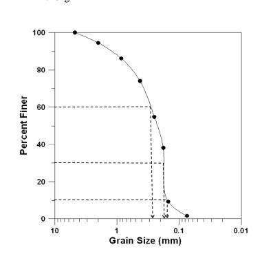
b.  $D_{10} = 0.17 \text{ mm}; D_{30} = 0.18 \text{ mm}; D_{60} = 0.28 \text{ mm}$
