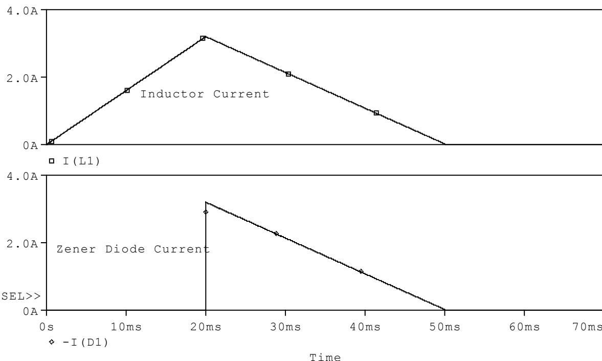
b) Power in the inductor is zero, but power in the  $1.5\Omega$  resistor is 1.76 W. Power absorbed by the Zener diode is 6.35 W. Power absorbed by the switch is 333 mW.
