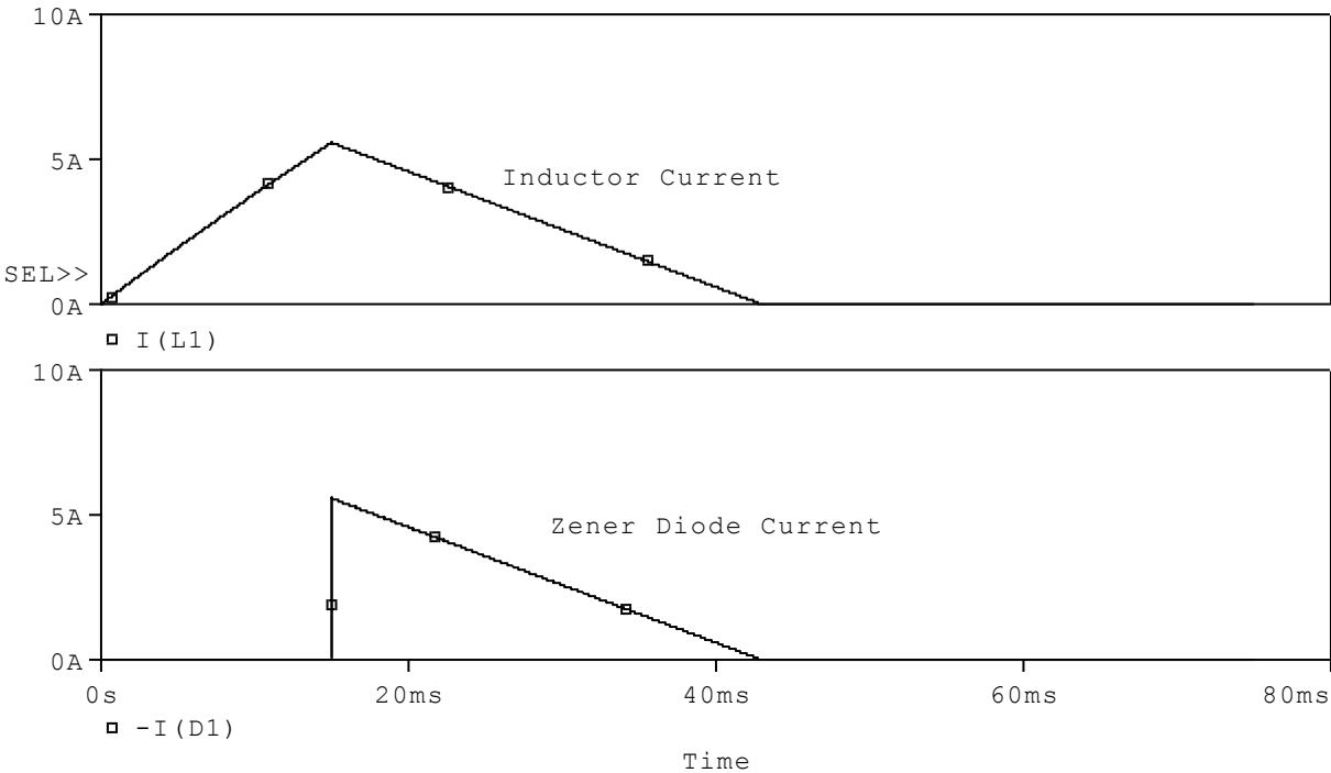
b) Power in the inductor is zero, but power in the  $1.5\Omega$  resistor is 4.4 W. Power absorbed by the Zener diode is 14.2 W. Power absorbed by the switch is 784 mW.
