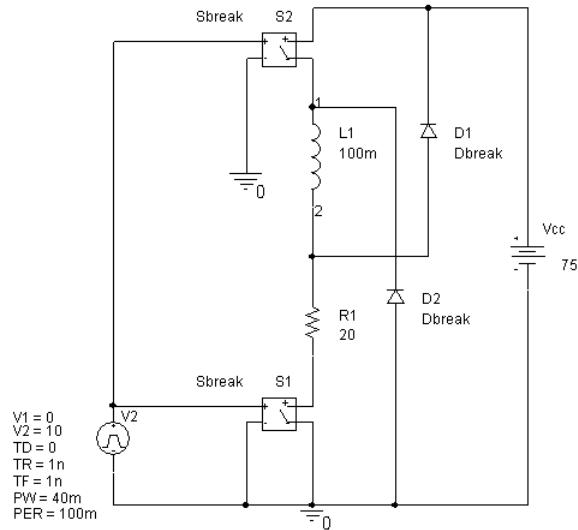
The inductor current reaches a maximum value of 3.4 A with the resistances in the circuit:  $I = 75/(20+1+1) = 3.4 \text{ A}$ .
