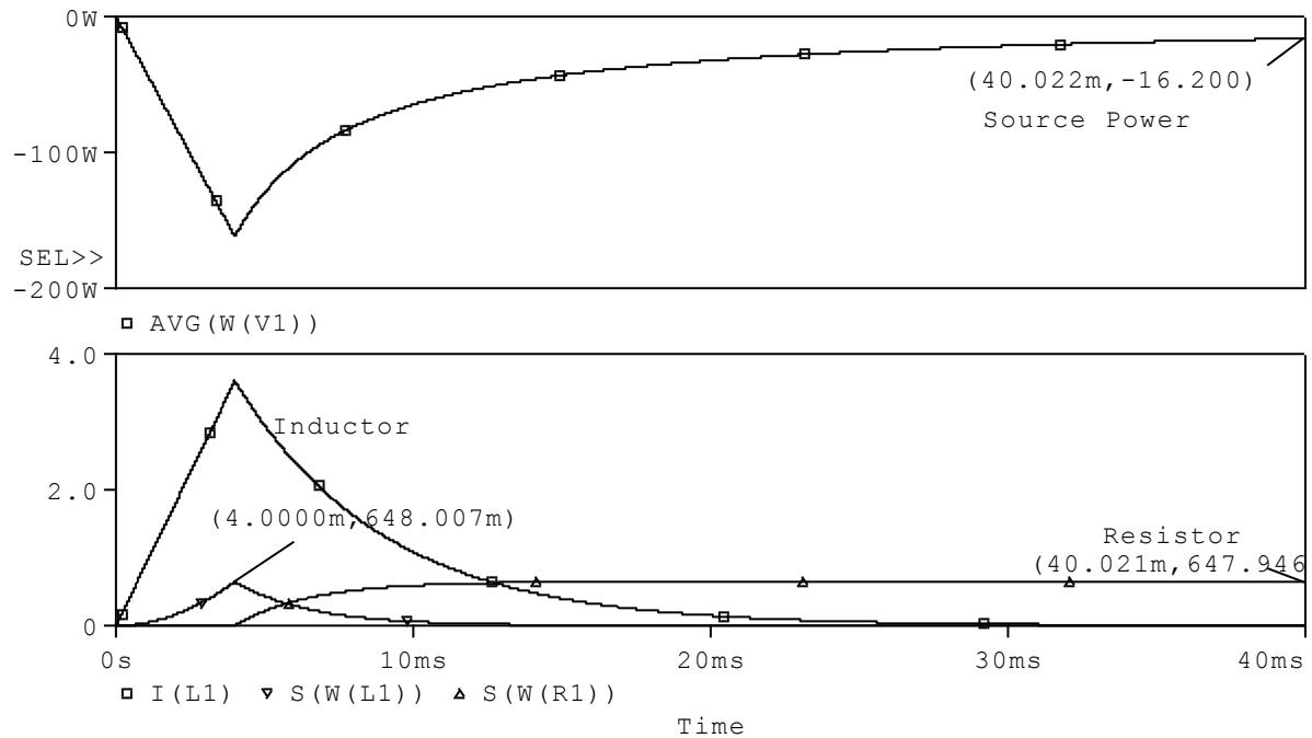
The inductor peak energy is 649 mJ, matching the resistor absorbed energy. The source power is -16.2 W absorbed, meaning 16.2 W supplied.
