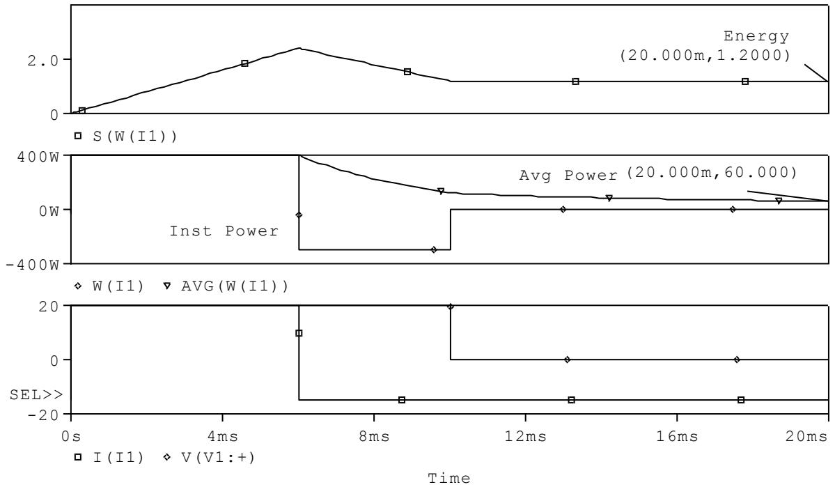
2-33) Average power for the resistor is approximately 1000 W. For the inductor and dc source, the average power is zero (slightly different because of numerical solution).
