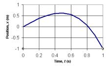
2. (b) Find the average velocity from t = 0.35  $v_{av} = \frac{\Delta x}{\Delta t} = \frac{\left[ (2 \text{ m/s})(0.45 \text{ s}) - (3 \text{ m/s}^3)(0.45 \text{ s})^3 \right] - \left[ (2 \text{ m/s})(0.35 \text{ s}) - (3 \text{ m/s}^3)(0.35 \text{ s})^3 \right]}{0.10 \text{ s}}$ to t = 0.45 s t = 0.45 s
