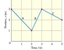
**Solution: 1. (a)** The magnitude of the slope at B is larger than A or C so we conclude the speed is greatest at B.
