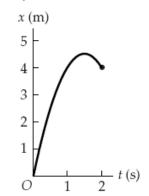
**Insight:** Note that the average velocity over the first second of time is equal to the slope of a straight line drawn from the origin to the curve at t = 1.0 s. At that time the position is 4.0 m.
