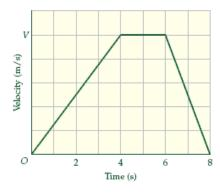
**Solution: 1. (a)** Determine the area under the curve by adding the area of the triangle from 0 to 4 s, the rectangle from 4 to 6 s, and the triangle from 6 to 8 s.
