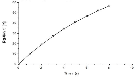
a. Since the two runners are running toward each other in exactly the same way, they will meet halfway between their respective starting points. That is, they will meet at x = 50.0 m. According to the graph, therefore, this position corresponds to a time of  $\boxed{6.6 \text{ s}}$ .
