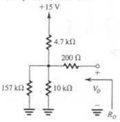
To obtain  $V_O=10.00~{\rm V}$  and  $R_O=3~{\rm k}\Omega$  we have to shunt both the 4.7-k $\Omega$  and the 10-k $\Omega$  resistors as shown. To yield an output voltage  $V_O=10.00~{\rm V}$  we must have
