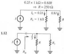
To make the current through R equal to L/3 we shunt R by a resistance  $R_1$  of value such that the current through it will be 2L/3; thus
