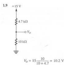
To reduce  $V_O$  to 10.00 V we shunt the 10-k $\Omega$  resistor by a resistor R whose value is such that 10 # R = 2 × 4.7.
