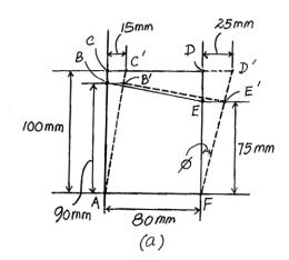
2-27. The material distorts into the dashed position shown. Determine the average normal strain that occurs along the diagonals AD and CF.
