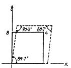
•2–25. The guy wire AB of a building frame is originally unstretched. Due to an earthquake, the two columns of the frame tilt  $\theta=2^{\circ}$ . Determine the approximate normal strain in the wire when the frame is in this position. Assume the columns are rigid and rotate about their lower supports.
