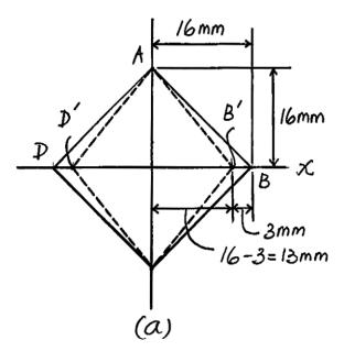
\*2-12. The piece of rubber is originally rectangular. Determine the average shear strain  $\gamma_{xy}$  at A if the corners B and D are subjected to the displacements that cause the rubber to distort as shown by the dashed lines.
