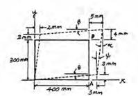
**2–19.** The piece of plastic is originally rectangular. Determine the shear strain  $\gamma_{xy}$  at corners D and C if the plastic distorts as shown by the dashed lines.
