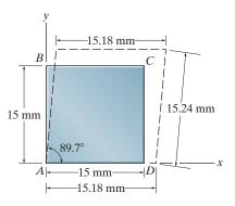
$$(\gamma_C)_{xy} = \frac{\pi}{2} - \left(\frac{89.7^{\circ}}{180^{\circ}}\right)\pi$$
