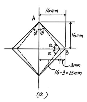
**2–11.** The corners B and D of the square plate are given the displacements indicated. Determine the average normal strains along side AB and diagonal DB.
