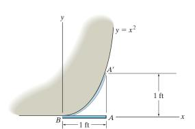
\*2–32. The bar is originally 300 mm long when it is flat. If it is subjected to a shear strain defined by  $\gamma_{xy} = 0.02x$ , where x is in meters, determine the displacement  $\Delta y$  at the end of its bottom edge. It is distorted into the shape shown, where no elongation of the bar occurs in the x direction.
