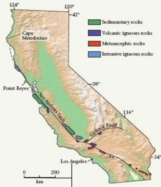
(b) Amount of fault movement indicated by offset bodies of identical rock.
