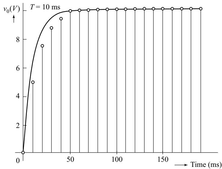
$$2.30 \text{ DT Model: } \frac{y[n+2] - 2y[n+1] + y[n]}{T^2} + \frac{5}{T} (y[n+1] - y[n]) + 6y[n] = x[n]$$
