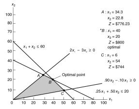
Changing the objective function to Z =\$16 $x_1$  + 16 $x_2$  would result in multiple optimal solutions, the end points being B and C. The profit in each case would be \$960.
