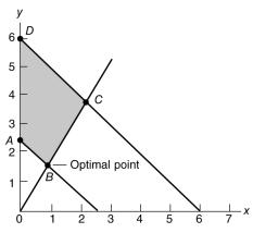
The optimal solution is x = 1, y = 1.5, and Z = 0.05. This means that a patrol sector is 1.5 miles by 1 mile and the response time is 0.05 hr, or 3 min.
