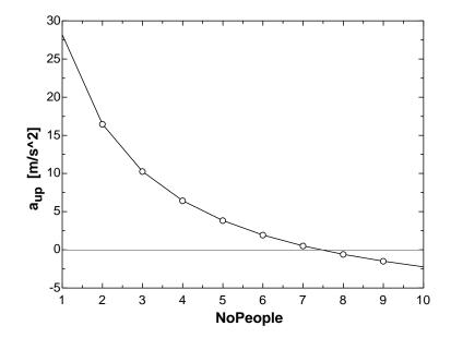
**2-92** A balloon is filled with helium gas. The maximum amount of load the balloon can carry is to be determined.
