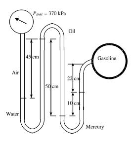
**2-104** A gasoline line is connected to a pressure gage through a double-U manometer. For a given reading of the pressure gage, the gage pressure of the gasoline line is to be determined.
