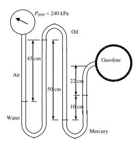
**2-105E** A water pipe is connected to a double-U manometer whose free arm is open to the atmosphere. The absolute pressure at the center of the pipe is to be determined.
