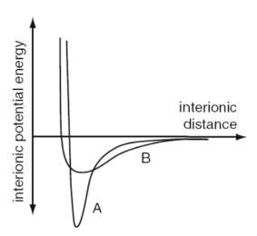
The well of titanium, represented by A, is deeper (higher melting point), has a larger radius of curvature (stiffer), and is more symmetric (smaller thermal expansion coefficient) than the well of aluminum, represented by B.
