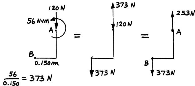
(b) From above figure: a 253-N upward force at A, and a 373-N downward force at B. ♦
