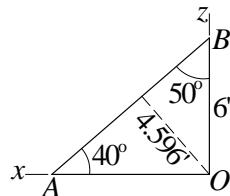
Note that only  $F_y = 71.55$  lb has a moment about  $AB$ . From trigonometry, the moment arm is  $d = 6 \sin 50^\circ = 4.596$  ft.
