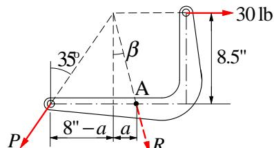
First find the direction of  $\mathbf{R}$  from geometry (the 3 forces must intersect at a common point).
