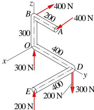
Split the 500-N force at  $D$  into the 200-N and 300-N forces as shown. We now see that the force system consists of three couples.
