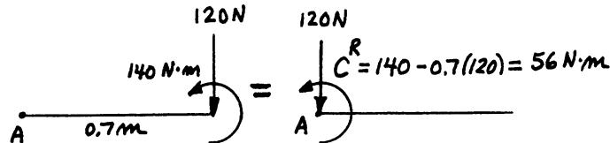
(a) From above figure: a 120-N downward force at A, and a 56 N·m CCW couple. ♦
