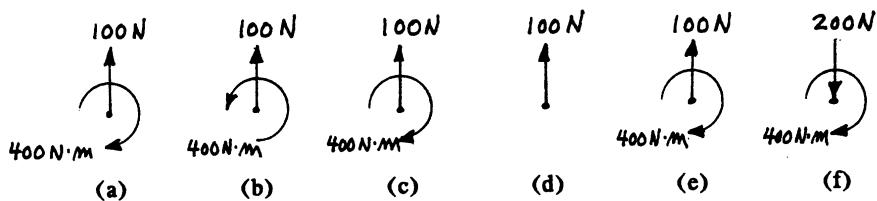
By inspection, the systems in (c) and (e) are equivalent to the system in (a). ♦
