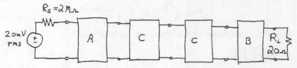
The cascade has R  $_{1}$  = 10 M $\Omega$ , R  $_{0}$  = 1  $\Omega,$  and A  $_{VO}$  = 376.9. The resulting loaded gain is
