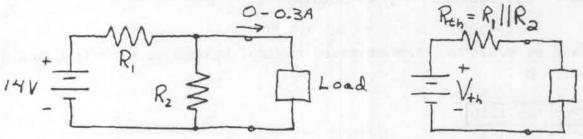
We denote the nominal values of the resistors as  $R_1$  and  $R_2$ . The highest load voltage (at most 6 V) occurs when  $I_L=0$ , when the resistor in parallel with the load has its highest value (which is  $1.05R_2$ ), and when the resistor in series with the source has its lowest value (which is  $0.95R_1$ ). To achieve the desired no-load voltage we need
