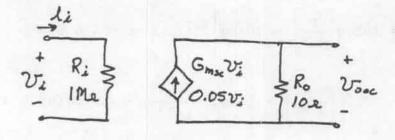
$$R_{\text{moc}} = \frac{v_{\text{ooc}}}{i_{i}} = \frac{G_{\text{msc}}v_{i}R_{o}}{v_{i}/R_{i}} = G_{\text{msc}}R_{o}R_{i} = 500 \text{ k}\Omega$$
