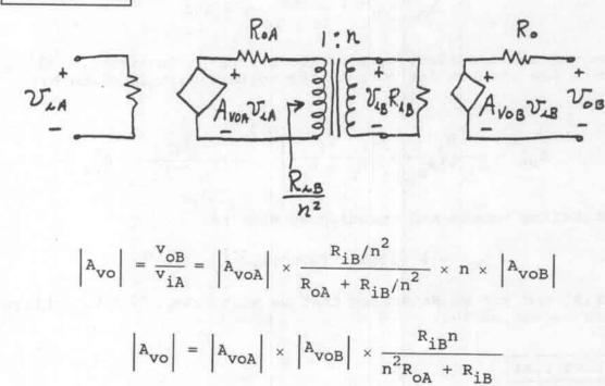
$$\frac{d|A_{VO}|}{dn} = 0 = \left|A_{VOA}\right| \times \left|A_{VOB}\right| \times \frac{R_{iB}^2 - n^2 R_{OA} R_{iB}}{(n^2 R_{OA} + R_{iB})^2}$$
