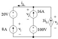
The voltage drop across the left branch, the center branch, and the right branch must be the same, since these branches are connected at the same two terminals. This requires that
