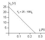
Note that when  $i_t = 0$ ,  $v_t = 25$  V; therefore the voltage source must be 25 V. Since the plot is a straight line, its slope can be used to calculate the value of resistance:
