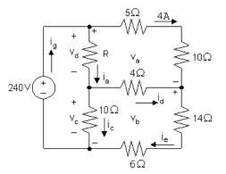
$$v_{a} = (5+10)(4) = 60 \text{ V}$$
