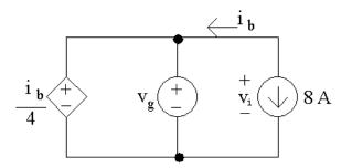
[a] Note that the current  $i_{\rm b}$  is in the same circuit branch as the 8 A current source; however,  $i_{\rm b}$  is defined in the opposite direction of the current source. Therefore,
