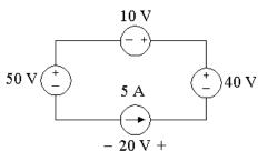
$P_{50V} = (50)(5) = 250 \text{ W} \text{ (abs)}$   $P_{10V} = (10)(5) = 50 \text{ W} \text{ (abs)}$   $P_{40V} = -(40)(5) = -200 \text{ W} \text{ (dev)}$   $P_{5A} = -(20)(5) = -100 \text{ W} \text{ (dev)}$   $\sum P_{dev} = 300 \text{ W}$
