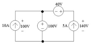
From the values of voltage and current in the figure, the power supplied by the current sources is calculated as follows:
