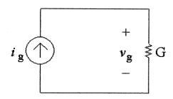
[a] Note from the circuit that the current through the conductance G is  $i_g$ , flowing from top to bottom, because the current source and the conductance are in the same branch of the circuit so must have the same current. The voltage drop across the current source is  $v_g$ , positive at the top, because the current source and the conductance are also in parallel so must have the same voltage. From a version of Ohm's law,
