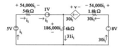
[a] To find  $i_1$ , write a KVL equation around the left-hand loop, summing voltages in a clockwise direction starting below the 5V source:
