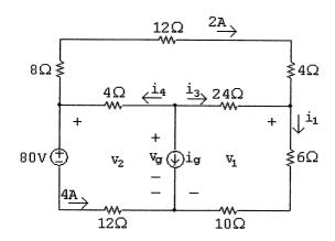
$$v_2 = 80 + 4(12) = 128 \text{ V};$$
