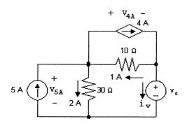
[a] To find  $v_s$ , write a KVL equation, summing the voltages counter-clockwise around the lower right loop. Start below the voltage source.
