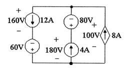
From the values of voltage and current in the figure, the power supplied by the currents sources is calculated as follows:
