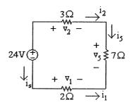
Write a KVL equation clockwise around the circuit, starting below the voltage source:
