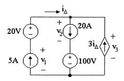
The voltage drop across the left branch, the center branch, and the right branch must be the same, since these branches are connected at the same two terminals. This requires that
