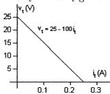
Note that when  $i_t = 0$ ,  $v_t = 25$  V; therefore the voltage source must be 25 V. Since the plot is a straight line, its slope can be used to calculate the value of resistance:
