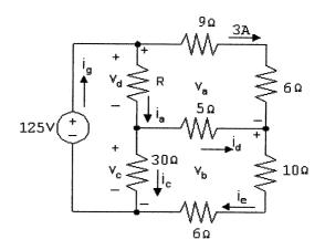
$$\begin{aligned} v_a &= (9+6)(3) = 45 \, \mathrm{V} \\ -125 + v_a + v_b &= 0 \quad \text{so} \quad v_b = 125 - v_a = 125 - 45 = 80 \, \mathrm{V} \\ i_e &= v_b/(10+6) = 80/16 = 5 \, \mathrm{A} \\ i_d &= i_e - 3 = 5 - 3 = 2 \, \mathrm{A} \\ v_c &= 5i_d + v_b = 5(2) + 80 = 90 \, \mathrm{V} \\ i_c &= v_c/30 = 90/30 = 3 \, \mathrm{A} \\ v_d &= 125 - v_c = 125 - 90 = 35 \, \mathrm{V} \\ i_a &= i_d + i_c = 2 + 3 = 5 \, \mathrm{A} \\ R &= v_d/i_a = 35/5 = 7 \, \Omega \end{aligned}$$
