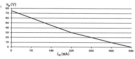
[b] Since the plot is linear for  $0 \le i_s \le 225$  mA amd since  $R = \Delta v/\Delta i$ , we can calculate R from the plotted values as follows:
