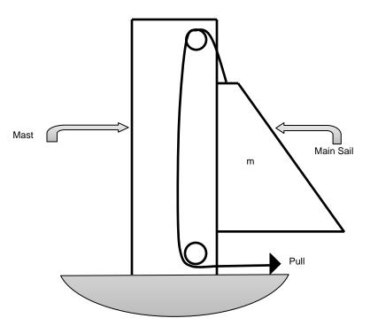
a. If the mainsail has a mass, m, and the pulleys are ideal (mass less and frictionless) how much pulling force must a crewmember exert to raise the mainsail at a constant speed? Explain.
