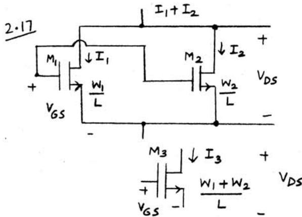
Note that all the transistors have equal terminal voltages so,
